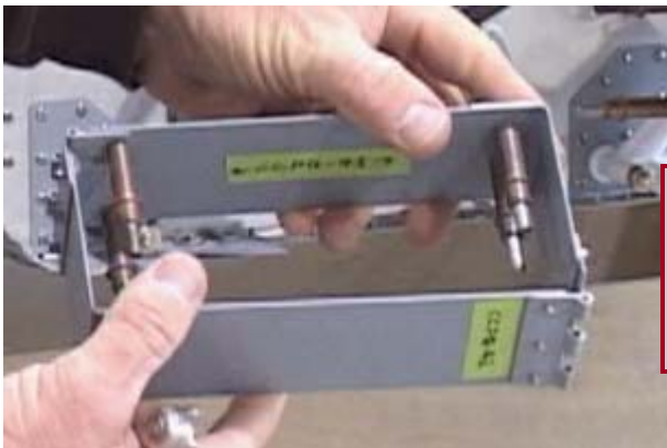
Fabricate battery clamp as shown from aluminum flat stock and piano hinge stock.
